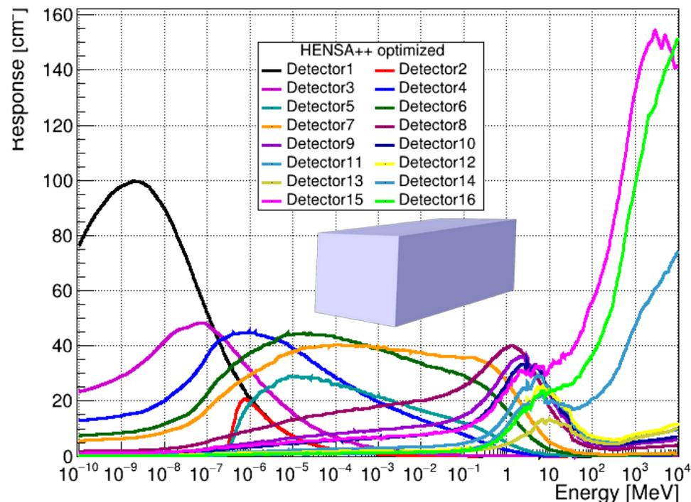
**HENSA** neutron response is **~10 times larger** than standard Bonner Spheres systems in the energy range from thermal up to 10 GeV.
