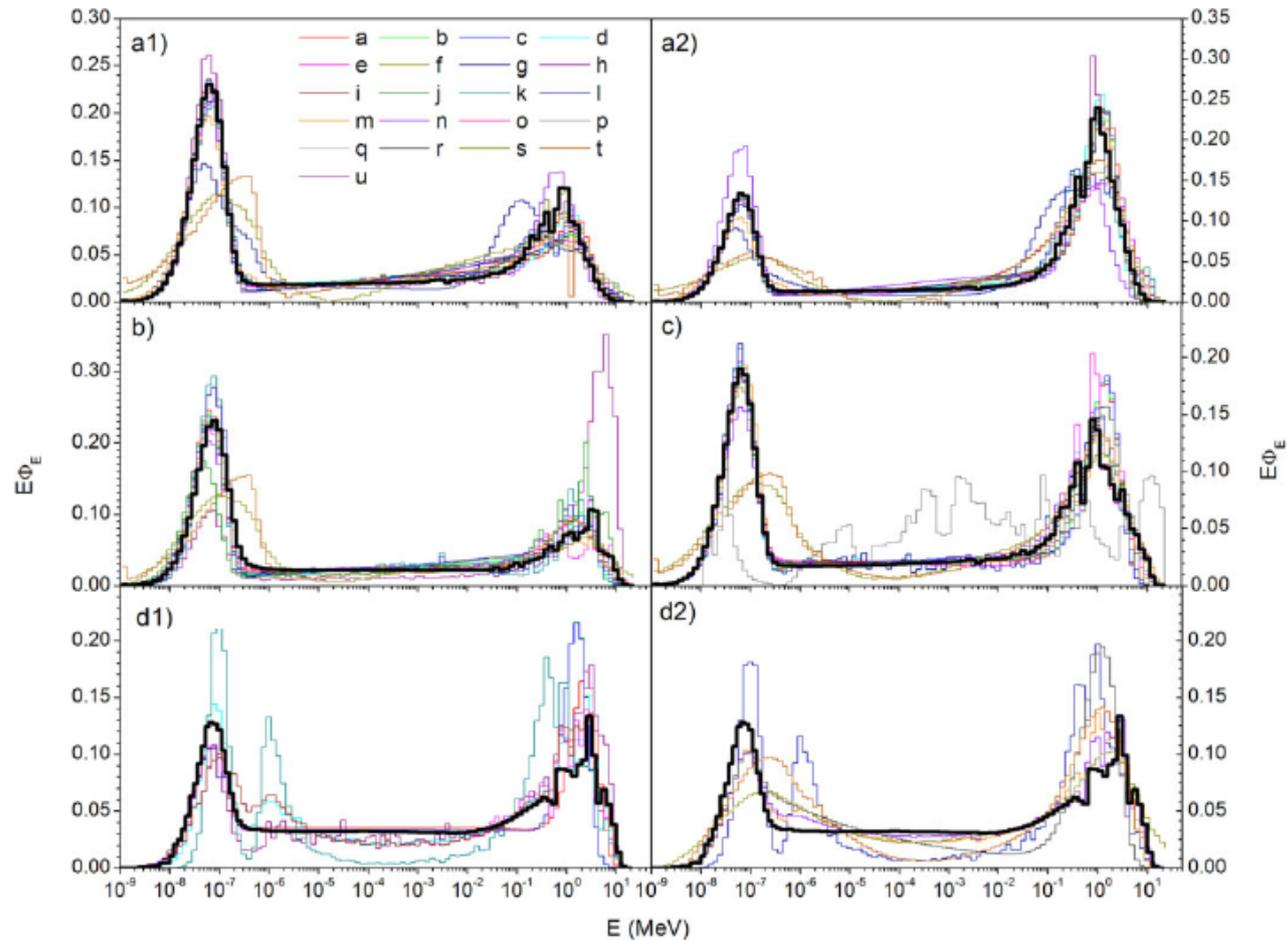
**Fig. 3:** Participants unfolded spectra (in colour) compared with the reference spectra for: a1) LINAC scenario, point 1 (at the entrance of the maze); a2) LINAC, point 2 (1 m from the isocentre); b) workplace; c) calibration facility; d) skyshine.
