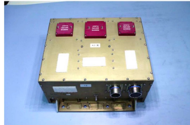
Fig. 8. SGPS instrument. Telescope apertures are under the “Remove Before Flight” covers.
