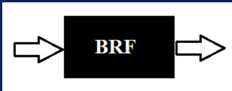
Band-Reject Filter (BRF) rejects the signals of a frequency band from 80 MHz to 120 MHz using Composite Right/Left-Handed (CRLH) elements.
