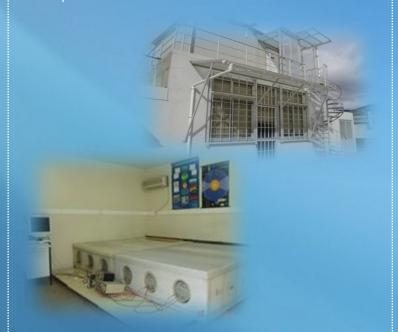
A.Ne.Mo.S. is housed in a specially constructed room at the roof of the Department of Physics at the campus of the NKUA. It consists of six BF3 gas proportional counters with the enriched isotope B type BP28 Chalk.
